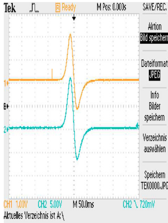
Figure 1 amplitude and phase signal of a metal ball 4mm Non-Ferrous. roughly corresponds to the behavior that the respective parts produce in a metal detector (300Khz) without product compensation.
